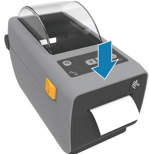
Press down on the front edge of the printer until it locks.
