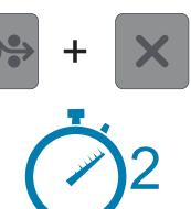
Press and hold the Feed (1) and Cancel (2) buttons for two seconds to print a configuration report.
