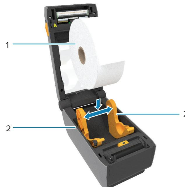
Spread the roll holders (1) open and place the roll (2) into the printer.
