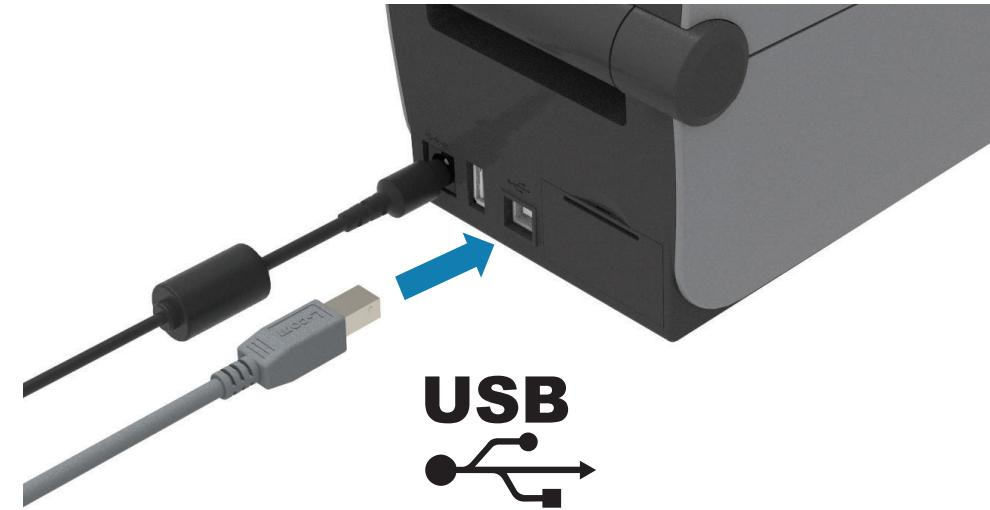
Connect a USB cable to the printer, connect the other end to your computer.
