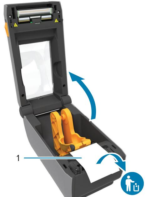
Open the printer and remove the packing (1).
