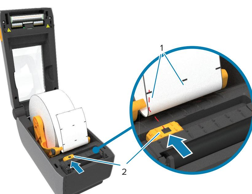
Align the sensor (2) to marks (1) away from the center of the roll for marked labels.
