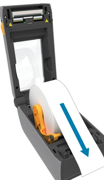
Pull the end of the roll past the front edge of the printer.
