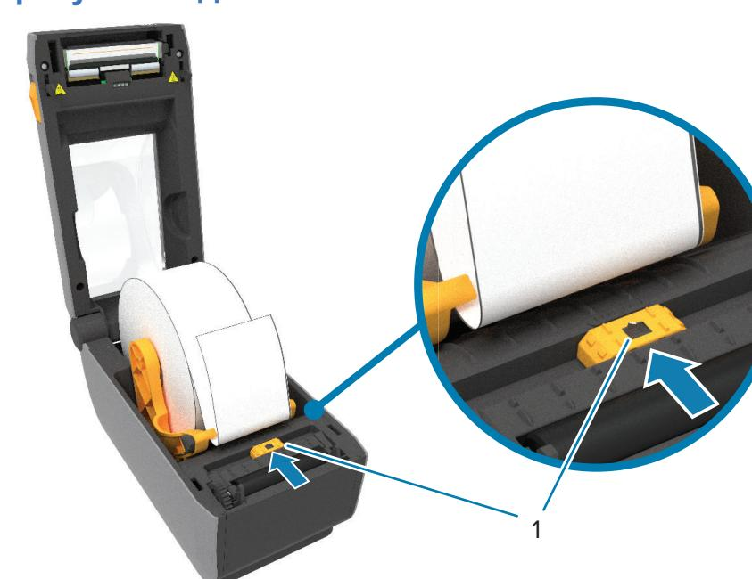
Align the sensor (1) to the center of the roll for regular labels and receipts.
