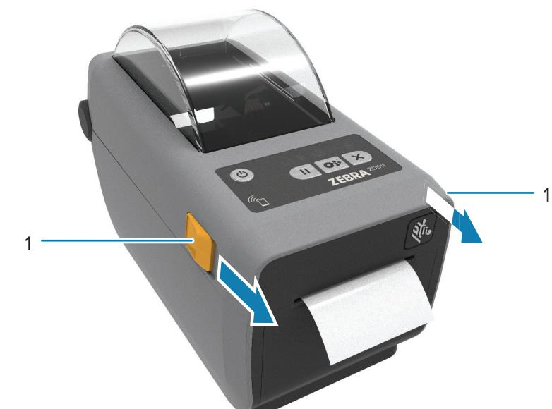
Slide the release latches (1) to the front to unlock the cover.
